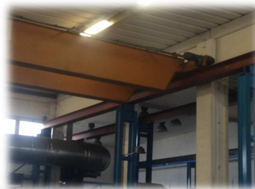
Bridge Crane for the production area with load capacity of 5 tons. Gauge 9 m
