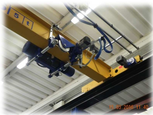
Bridge Crane for the production area with load capacity of 5 tons. Gauge 9 m
